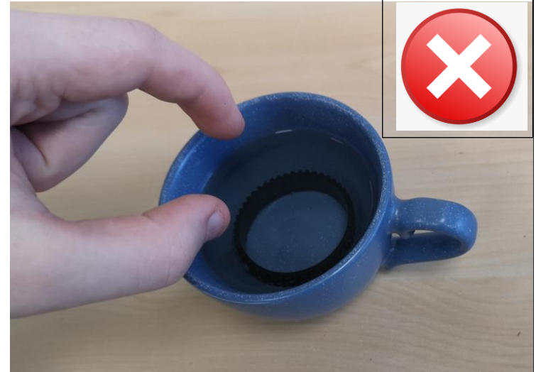
Don't use fingers to take braking lining out
