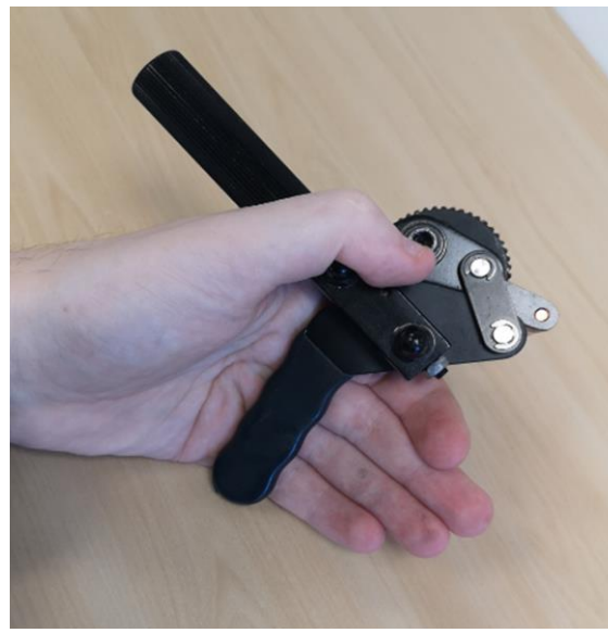
To be safe at cutting please hold brake as on the picture
