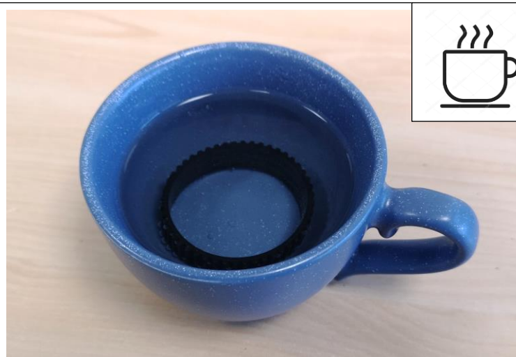
Put replacement braking lining in hot water (80°C) for 10 min
